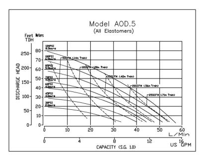
The performance curves shown and other published literature reflect an average performance for all materials and all elastomers, including Teflon®. Derating of the performance is not necessary for Teflon® fitted pumps.
